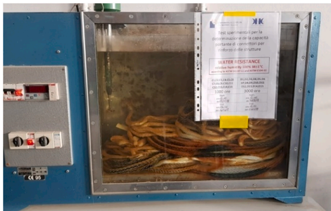
Fig. 12. Equipment for water environment at controlled humidity.
