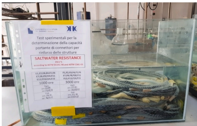
Fig. 11. Equipment for saltwater environment.
