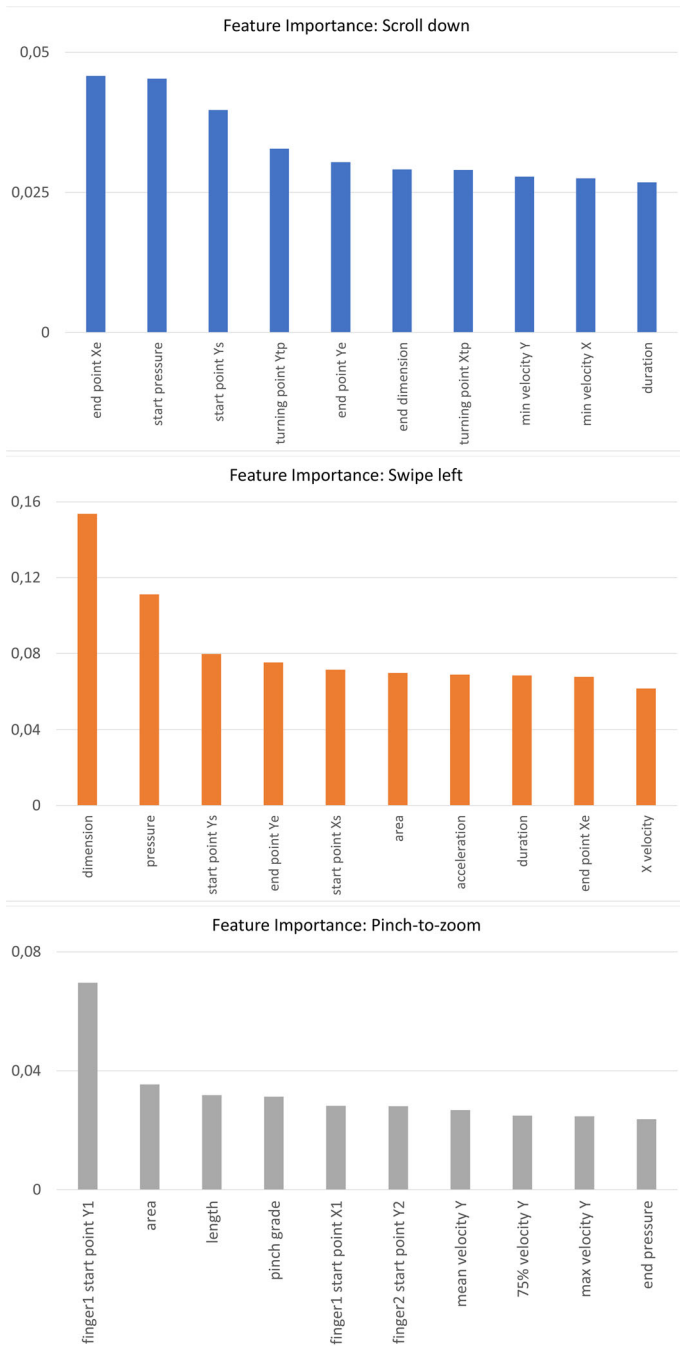
Fig. 5 The 10 most relevant features for scroll down, swipe right and pinch-to-zoom datasets, selected by Random Forest classifier
