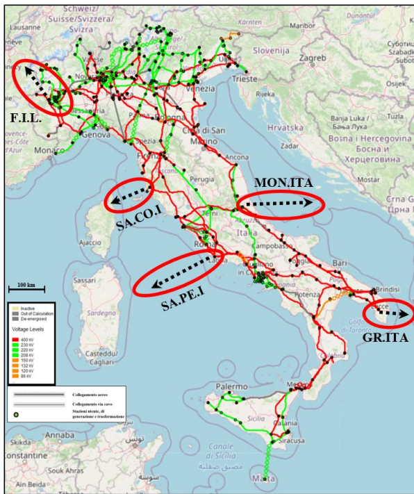
FIGURE 10. The Italian AC/DC network: the dotted arrows represent the HVDC links.
