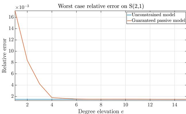
**FIGURE 6:** Integrated inductor. Relative error  $\epsilon_{2,1}$  for different degree elevation levels  $e$ . The blue line reports the corresponding error for a model generated without enforcing any passivity constraint.
