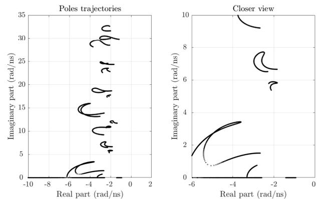
**FIGURE 12:** Parameterized poles trajectories of the coupled transmission line model. Left panel: in-band poles. Right panel: enlarged view on the low-frequency region.
