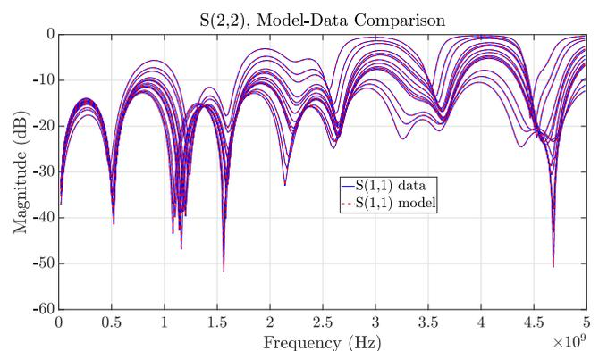
**FIGURE 16:** High-speed link. Comparison of model responses ( $e = 25$ ) with the corresponding raw data over a random subset of 14 out of the total 81 available frequency responses.
