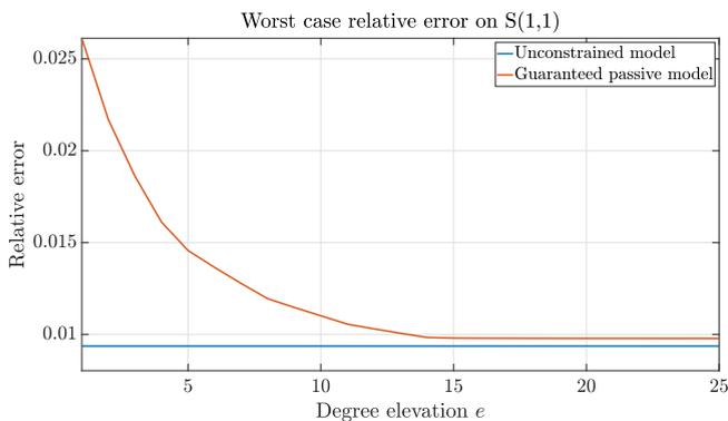
**FIGURE 17:** High-speed link. Evolution of the relative error index  $\epsilon_{1,1}$  for the passive models with different degree elevations, compared to the unconstrained model error.
