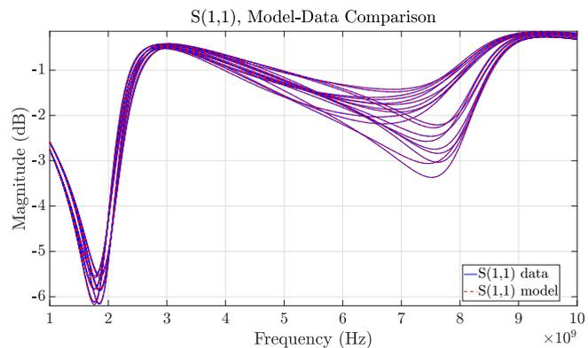
**FIGURE 19:** LNA example. Comparison between model responses and validation data over 19 different frequency responses, randomly selected in the design space.
