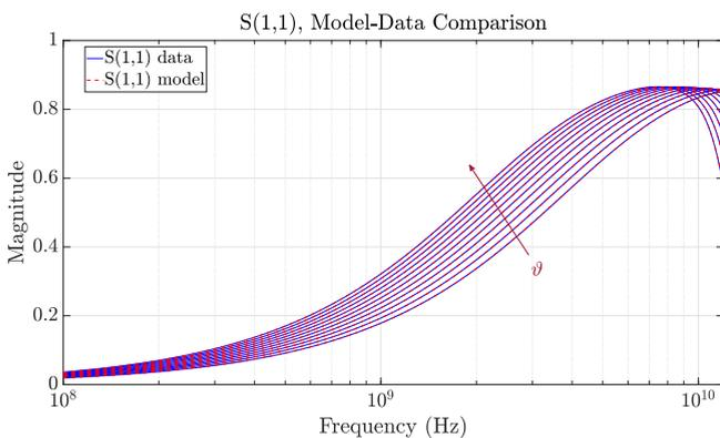
**FIGURE 5:** Integrated inductor. Comparison between parameterized model responses and training data for a degree elevation level  $e = 50$ ; all the  $\bar{m} = 11$  parameter configurations are shown.
