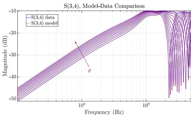
**FIGURE 10:** Coupled transmission line. Fitting of the responses magnitude of the  $S(3, 4)$  transfer function element.
