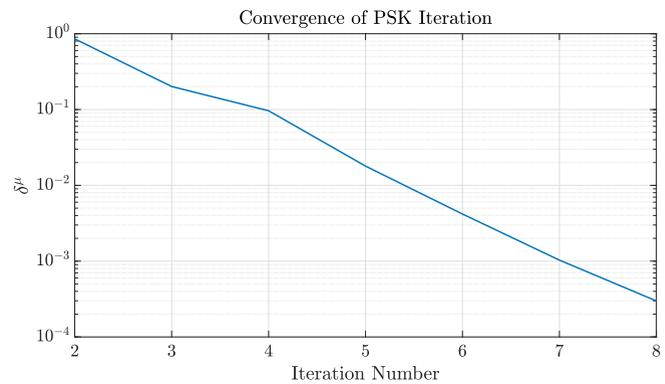
**FIGURE 7:** Coupled transmission line. Evolution of the convergence index  $\delta^\mu$  through iterations.
