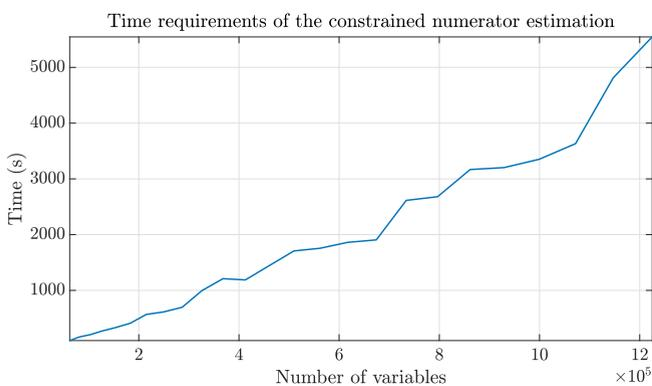
**FIGURE 14:** High-speed link. Time required to enforce the model passivity, as a function of the number of variables required by different degree elevation levels.
