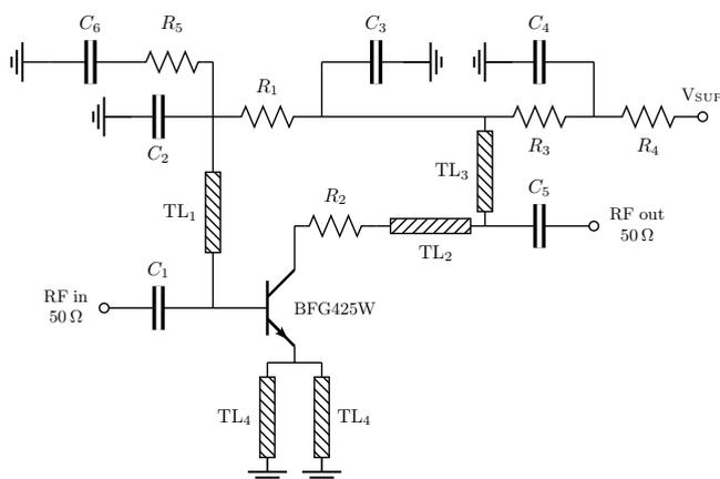
**FIGURE 18:** Schematic of a parameterized LNA.
