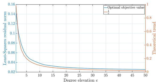
**FIGURE 3:** Integrated inductor. Residual norm of the constrained numerator coefficients estimation problem, as a function of the degree elevation level  $e$ . The experimental results are compared to a reference asymptotic  $1/e$  trend, which is expected based on the theory [36].
