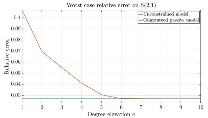
**FIGURE 11:** Coupled transmission line. The relative error  $\epsilon_{2,1}$  for the passive models based on different degree elevations, compared to the error of the model obtained without enforcing any passivity constraint.
