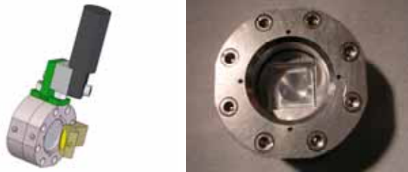
Figure 6. Cerenkov converter vacuum-tight holder, for containment of aerogel, with upstream entrance foil and downstream quartz window.
