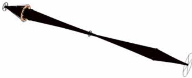
Figure 11. Optical transport line, with 5 % bandpass filter centered on 800 nm. Aerogel index of refraction n = 1.0084 .
