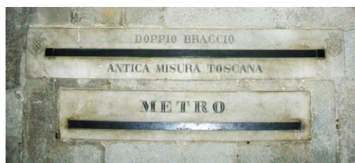
Figure 4. The lengths of the metre and of the double cubit ( doppio braccio ) on the walls of the town hall in Pistoia. The inscription indicates that the double cubit (120 cm long, so giving a 60 cm long cubit) is an ancient Tuscan measure.
