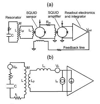
FIG. 1. (a) Schematic circuit diagram of the two-stage dc SQUID coupled to the high-Q resonator. (b) The dc SQUID is modeled by an ideal current amplifier with the noise sources  $V_n$  and  $I_n$ . The real part of the dynamic input impedance is represented for convenience by the cold resistor  $r_c$  in series to the resonator.
