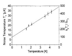
FIG. 3. Approximate noise temperature  $T'_n = [S_{vv}(\omega_0)S_{ii}(\omega_0)]^{1/2}/2k_b$  at  $\nu_0 = 1671$  Hz. The continuous line is the best linear fit to the data.
