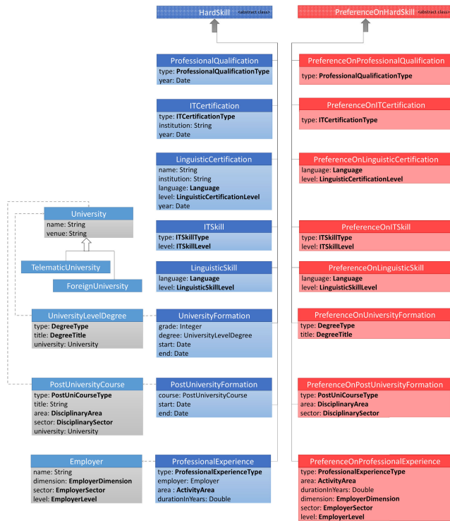
FIGURE 5. The classes defined for modelling employees' hard skills and the preferences of managers on that type of skill.
