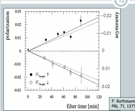
Spin filtering works for protons
