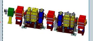
Installation of six magnets for the low-B insertion
