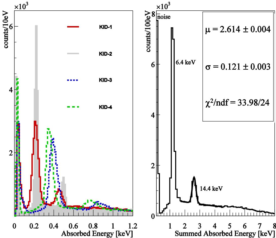
energy conversion efficiency to break cooper pairs  $\eta = 2.6/14.4 = 18\%$
