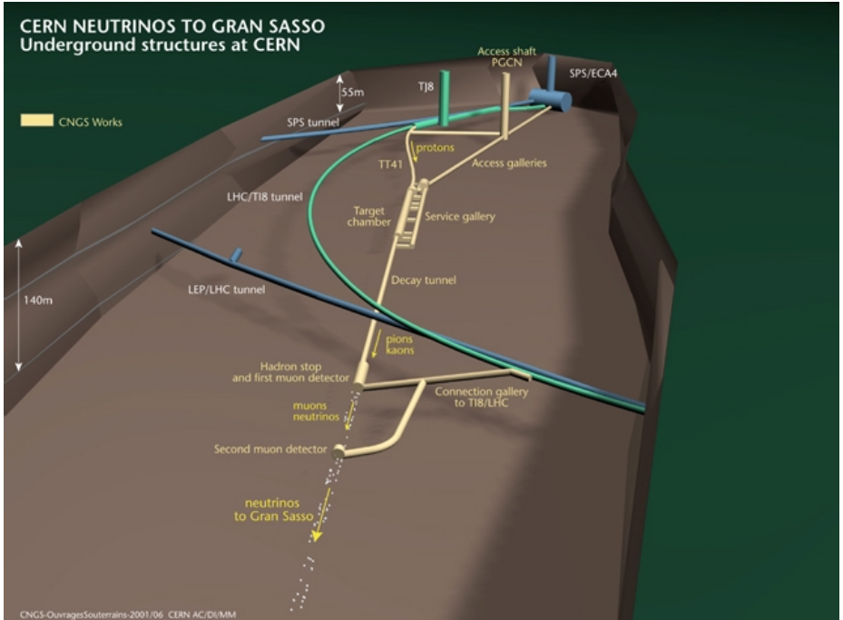
Fig. 11. Underground layout of the CNGS neutrino beam from CERN to Gran Sasso
