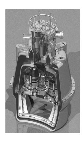
Figure 2. The cut-away 3D view of the ZEPLIN-II central detector.
