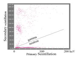
Figure 1. Secondary vs primary scintillation in two-phase Xe with mixed gamma and neutron sources. The secondary scintillation photons are produced by an electroluminescent process in gaseous Xe.
