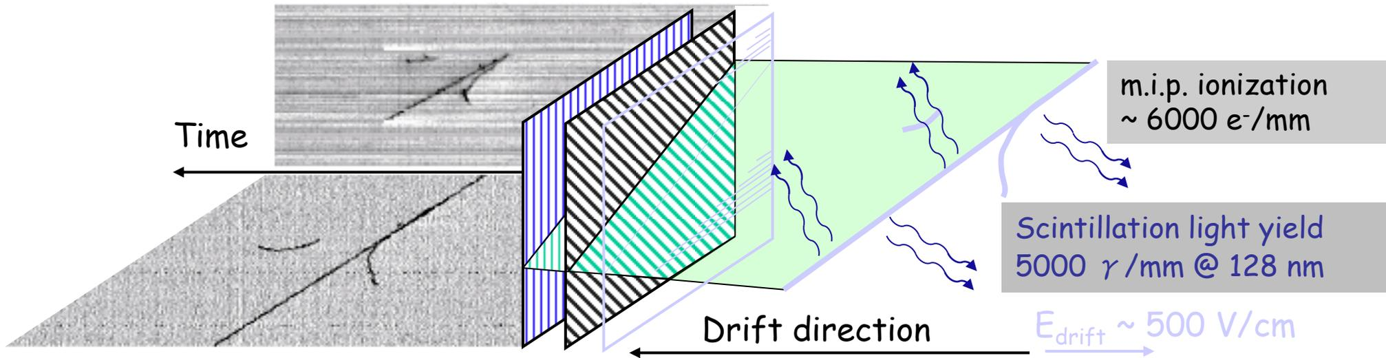
Electrons from ionizing track are drifted in LAr by  $E_{\text{drift}}$ . They traverse transparent wires arrays oriented in different directions where induction signals are recorded. Finally electron charge is collected by collection plane.
