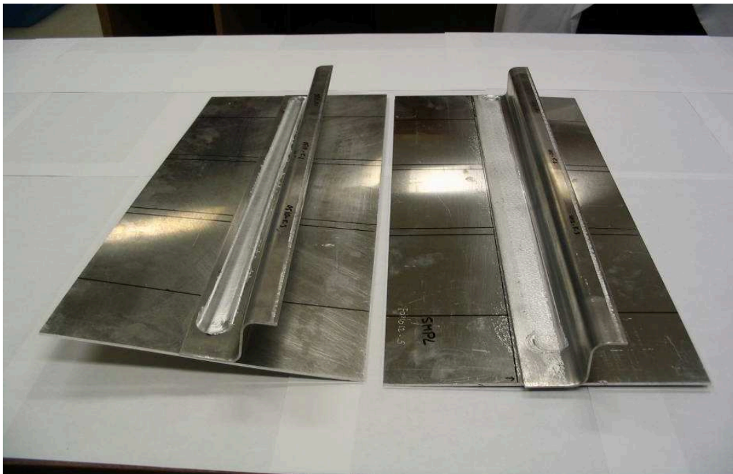
Figure 1: FSW plate before and after hammer peening [2]
