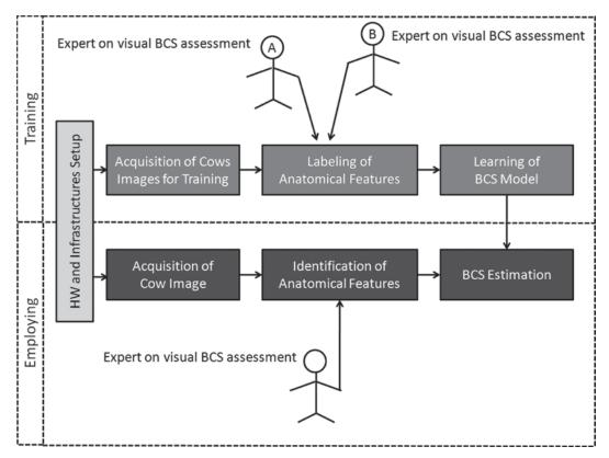
Figure 1. The scheme of a system for semiautomatic estimation of BCS. HW = hardware.
