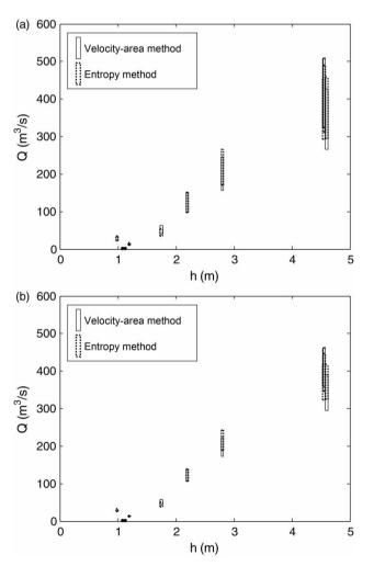
Figure 9 | Equipped section – Ponte Felcino: comparison between the grey discharges estimated through the velocity-area method grevified (a) through the type I approach and (b) through the type II approach, with the corresponding grey discharges estimated through the grey entropy method.
