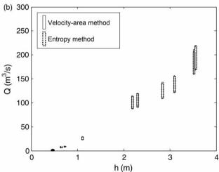
Figure 10 | Equipped section – Santa Lucia: comparison between the grey discharges estimated through the velocity-area method greyified (a) through the type I approach and (b) through the type II approach, with the corresponding grey discharges estimated through the grey entropy method.
