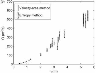
Figure 8 | Equipped section – Ponte Nuovo: comparison between the grey discharges estimated through the velocity-area method grevified (a) through the type I approach and (b) through the type II approach, with the corresponding grey discharges estimated through the grey entropy method.
