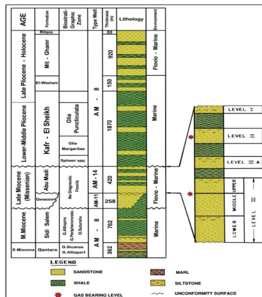
Fig. 3: Stratigraphic Column and Reservoir Zonation of AM/EQ Fields (El Heiny et al. , 1990).
