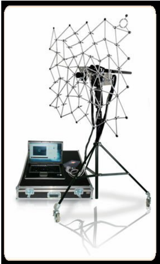
Figure 2: Pseudo random microphone array used for the measurements
