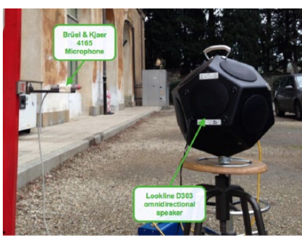
Figure 3. Setup for the noise source characterization
