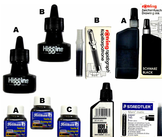
Fig. 1. India ink used for measurements. Samples are from five different brands (Higgins, Rotring, Pelikan, Staedtler, and Koh I Noor) and for some brands also from different batches (three batches of Pelikan, two of Higgins, and two of Rotring).
