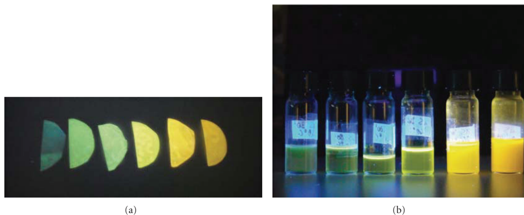
FIGURE 1: CdS nanoparticles (a) inside the polystyrene matrix and (b) in chloroform after the polymer removal. The reported samples were obtained heating a polymer/precursor foil at 300°C for 2, 5, 10, 15, 20, and 30 min (from left to right) when different colors of the samples indicate QDs with different sizes.
