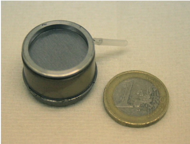
Fig. 10 A bare MXS source, without source holder and LEDs, showing the size, next to a 1€ coin, for comparison. The top of the source shows the beryllium exit window.
