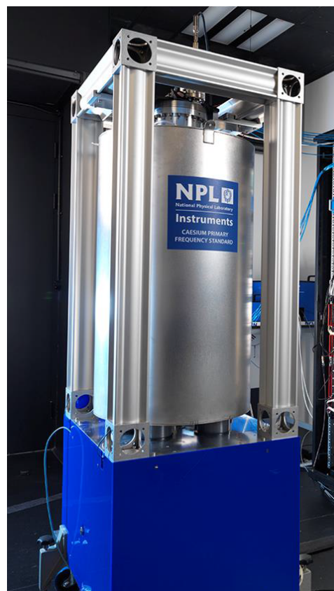
Fig. 1. Photograph of the AOS-CsF1 physics package — the first of the new NPL design to be assembled.
