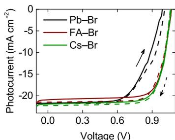
**Figure 2.** Experimental results for three PSCs. (a)  $J-V$  characteristics for forward (solid line) and reverse (dashed line) scans. Black, red, and green lines represent PSCs with  $\text{Pb-Br}$ ,  $\text{FA-Br}$ , and  $\text{Cs-Br}$  bromide sources, respectively.
