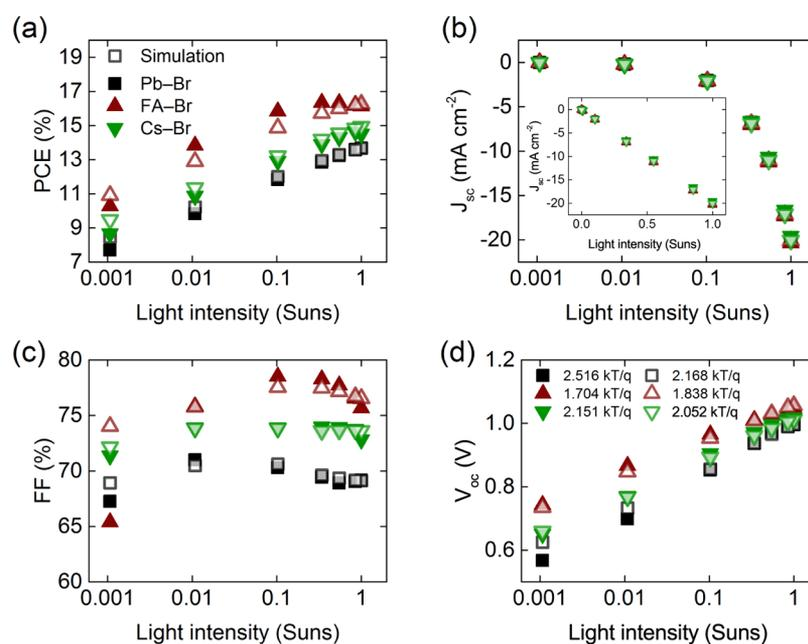
**Figure 6.** Photovoltaic experimental (full symbol) and simulation (open symbol) results for different illuminations: (a) PCE, (b)  $J_{sc}$  with inset having linear scale, (c) FF, and (d)  $V_{oc}$ . Solar cell structure with Pb–Br (square symbol), FA–Br (up triangle symbol), and Cs–Br (down triangle symbol) bromide source. The parameters used for simulation are shown in Table 2. 1 sun = 100 mW cm<sup>-2</sup>.
