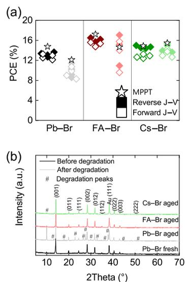
**Figure 5.** Experimental results for the degradation effect: (a) PCE and (b) XRD results. Fresh (dark color) and 9 months old (greyish color) samples. Perovskite with Pb–Br (black), FA–Br (red), and Cs–Br (green) sources of bromide.
