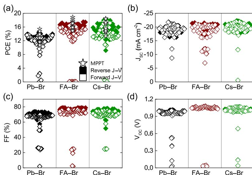
**Figure 1.** Photovoltaic parameters for PSCs with the effect of different bromide sources, (a) PCE, (b)  $J_{sc}$ , (c) FF, and (d)  $V_{oc}$ . Perovskites with Pb-Br (black points), FA-Br (red points), and Cs-Br (green points) as the sources of bromide.
