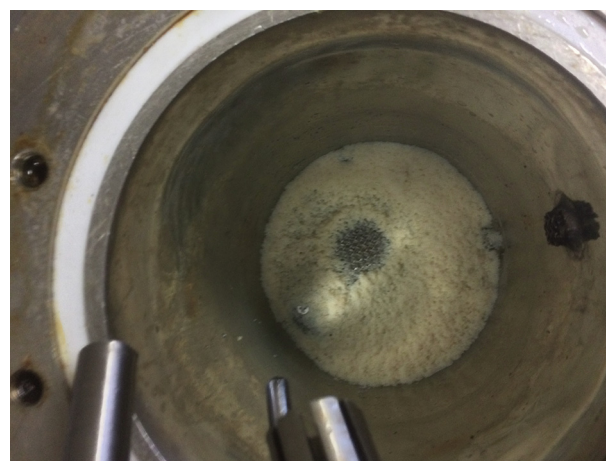
Fig. 6. Combined effects of ultrasonic irradiation and emulsification in the bed of immobilized PS lipase inside the batch reactor.
