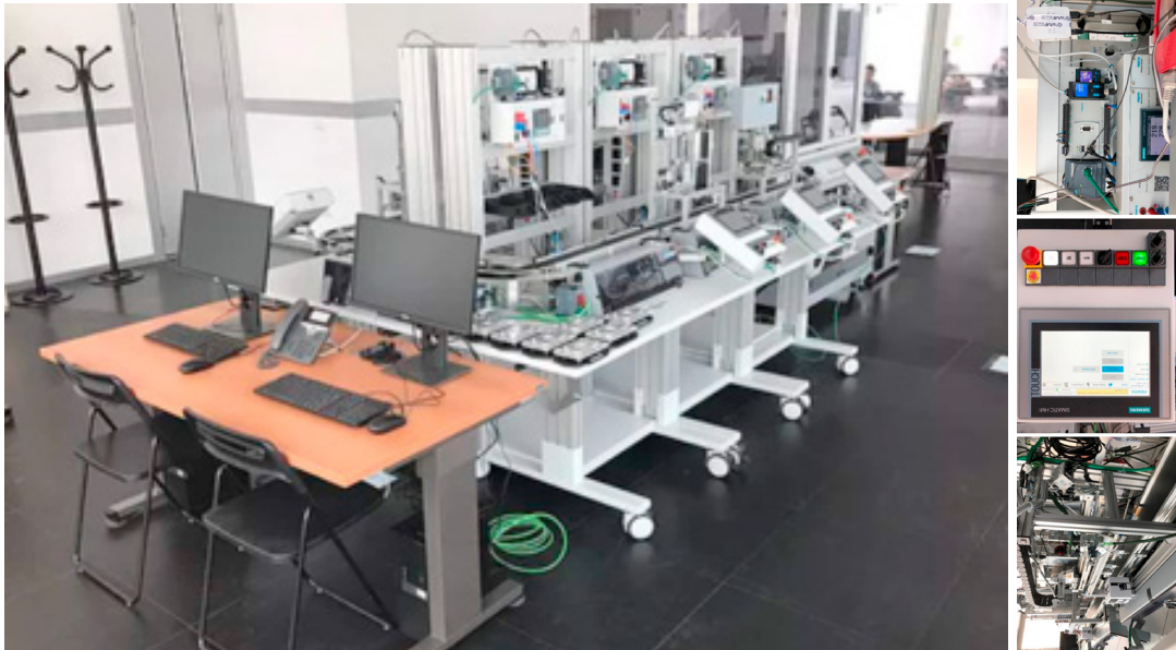
Figure 1. Picture of the modular smart manufacturing system we used with close ups on the right-hand side.
