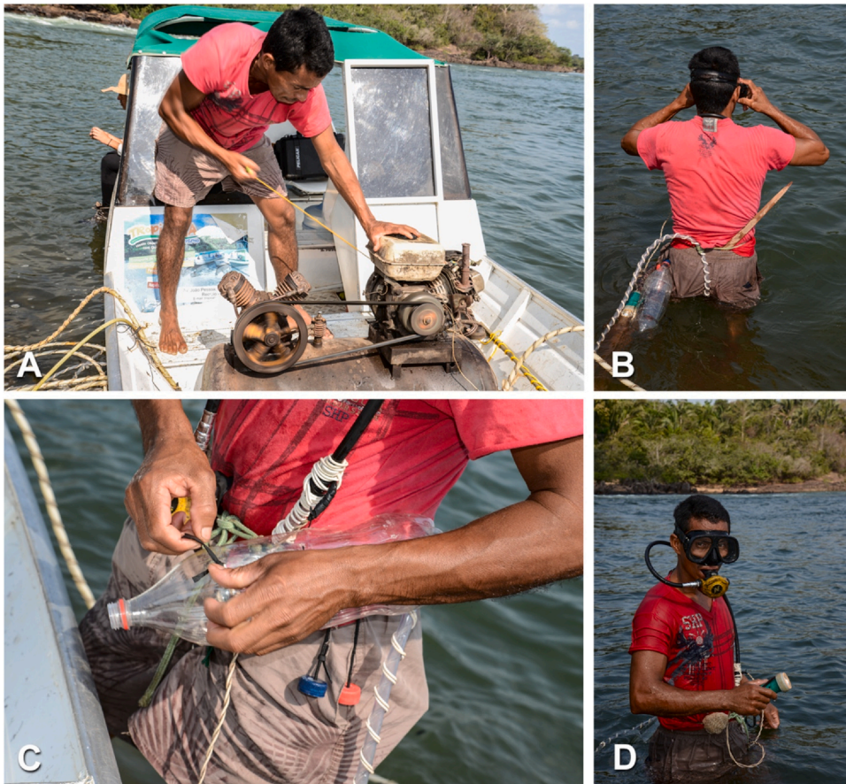
Fig. 5. The hookah diving equipment used by the “acarizeiros”. A) A homemade air-compressor; B) Fisherman adjusting his dive mask and air-hose. The bottles are attached to his belt. He also carries a wooden stick (called “vaqueta”) to coax the fish from the crevices; C) Soda bottle being prepared to hold the fishes captured during the dive; D) Acarizeiro ready to go fishing. Photographs by L. Sousa.
