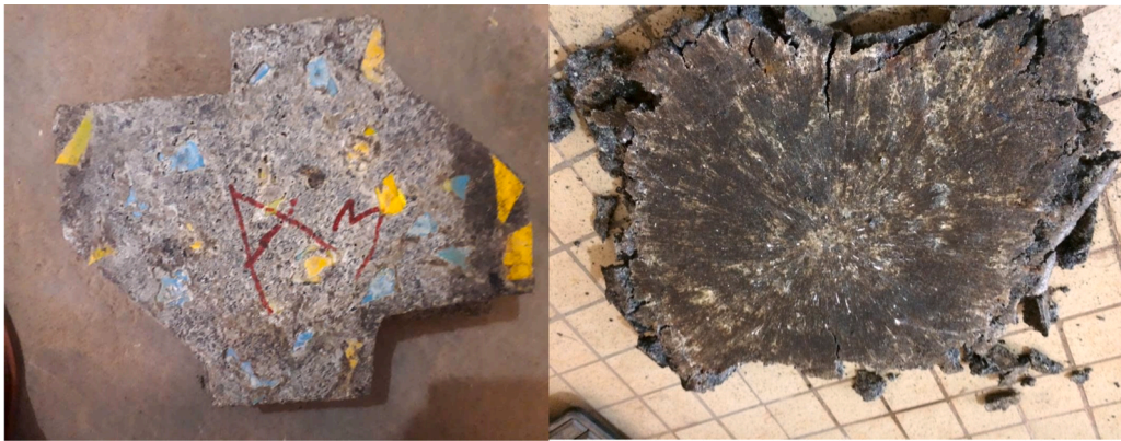
a) MPB-pavers before (left) and after (right) compressive strength tests
