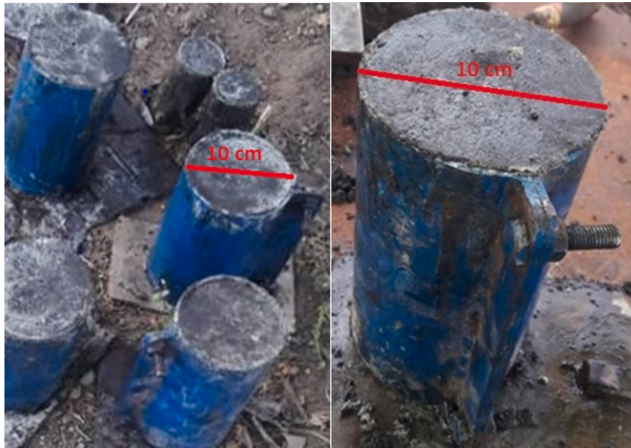
Fig. 4. Samples of MPB with melted plastic wastes as binder.
