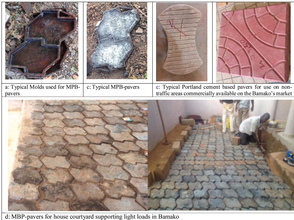
Fig. 12. (a) Used steel moulds for the MPB-pavers, (b) typical interlocking block pavers made from MPB, (c) typical Portland cement-pavers on sale on the Bamako's market, and (d) an example of house courtyard in Bamako with interlocking MPB-pavers.
