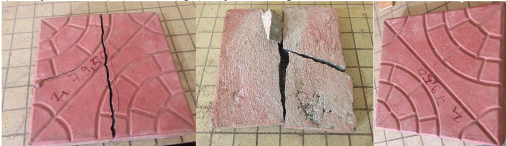
b) Portland cement-based pavers from the Bamako's market before (right) and after (left) compressive strength tests
