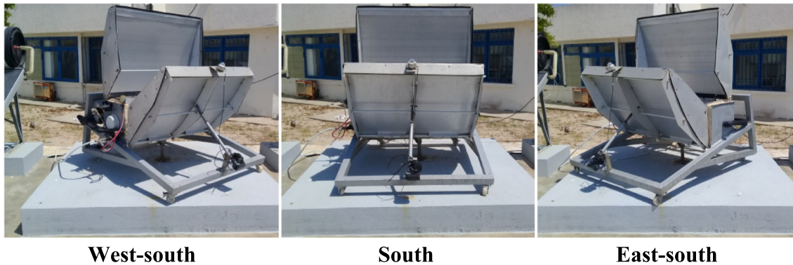
FIGURE 4 Integrated solar storage collector system orientations toward south, east-south, and west-south (a mobile support) [Colour figure can be viewed at wileyonlinelibrary.com]
