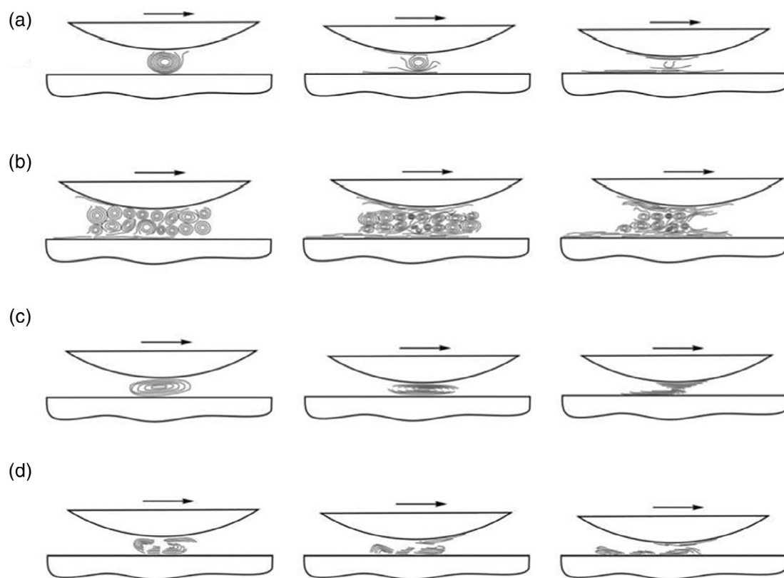
FIGURE 5 Schematic presentation of the various mechanical routes for the exfoliation process: (a) individual exfoliation of nanotubes; (b) exfoliation of aggregate nano-sheets; (c) exfoliation of nanotubes; (d) breaking of nanotubes and exfoliation of smaller, broken multi-wall pieces. The sliding direction is shown by the arrows, reproduced with authors permission and copyrights holder of Ref. 108
