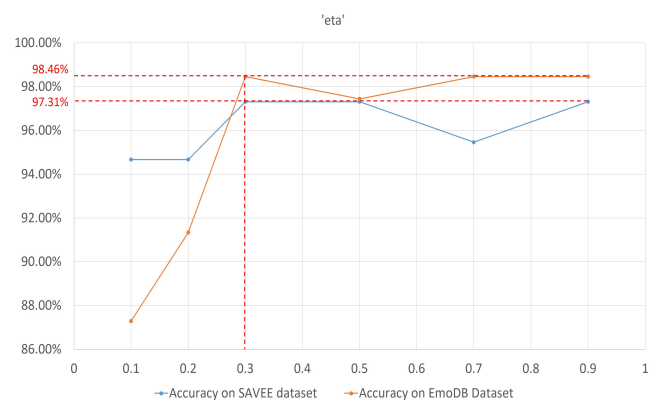
FIGURE 13: Variation of accuracy with respect to 'eta' value for both SAVEE and EmoDB datasets
