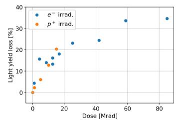
**Figure 4.** Percentage light yield loss after electron and proton irradiations as a function of the delivered dose measured upon excitation with a <sup>137</sup>Cs source.
