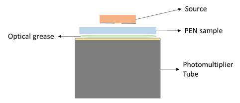
**Figure 2.** Schematic representation of the experimental setup for the PEN thin-film scintillator's light yield measurement.
