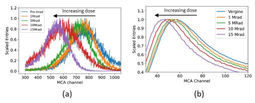
**Figure 3.** Light yield spectra of proton irradiated thin-film PEN scintillators excited by (**a**) alpha particles from a <sup>241</sup>Am source and (**b**) electrons from a <sup>137</sup>Cs source.
