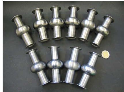
Figure 12: 6GHz cavities made of Nb (in the upper part) and V (in the bottom part).
