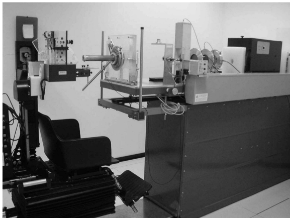
Figure 1. The proton therapy beam line for the treatment of ocular melanoma, installed at Laboratori Nazionali del Sud - INFN in Catania, Italy.
