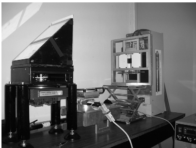
Fig. 10. Photo of the wide field laboratory CT system.
