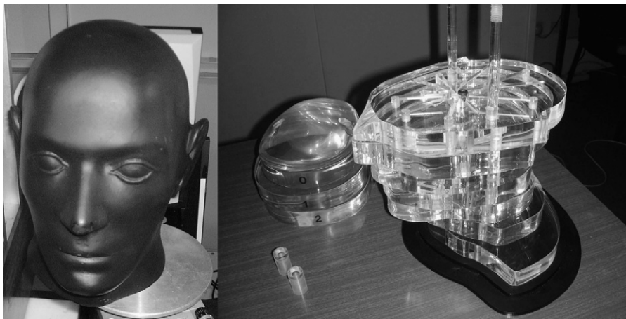
Fig. 1. Left: human head with anatomy inserts; right: calibration phantom.
