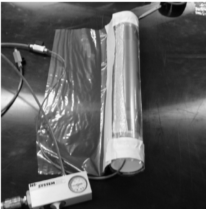
Fig. 1. A cylindrical GEM foil realized with vacuum bag technology.
