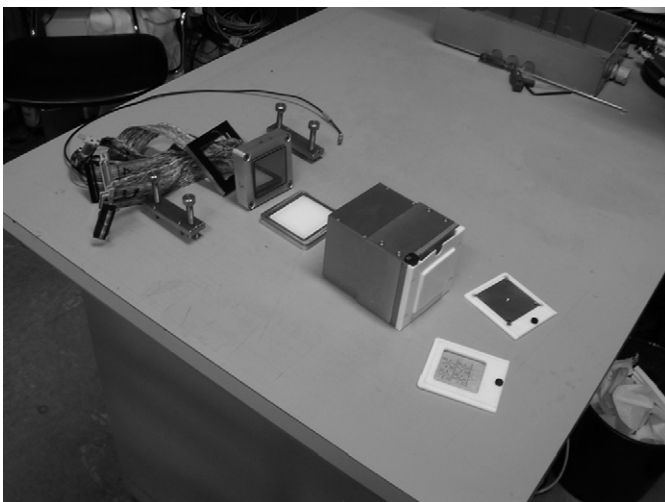
Fig. 1. One of the detector systems used, based on a flat panel PSPMT. Collimation masks can be seen to the right of the detector box.
