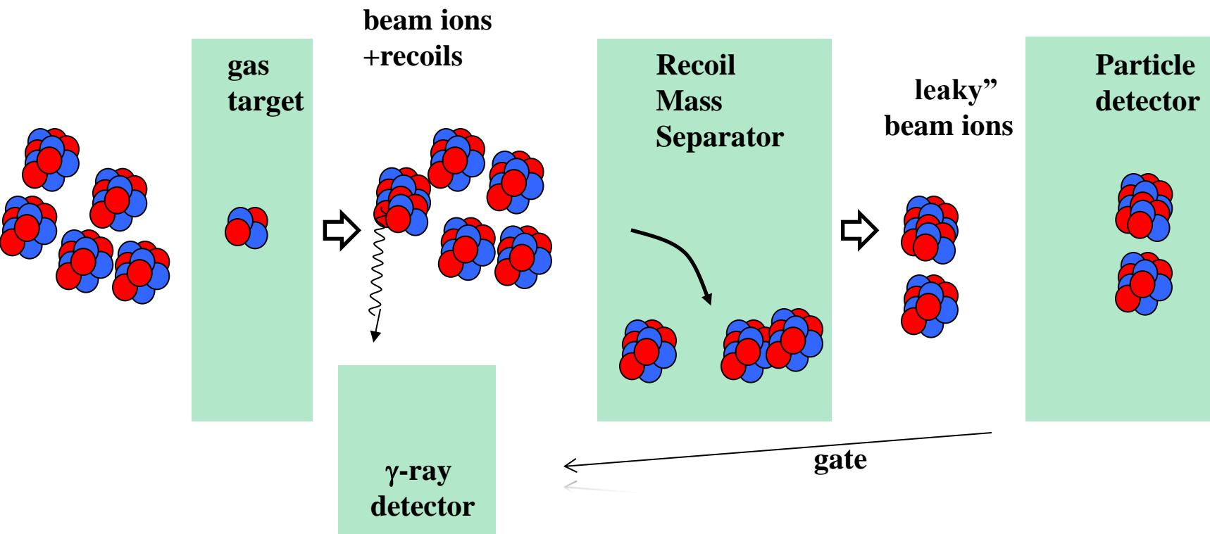
$$N_{\text{recoils}} = N_{\text{projectiles}} \times n_{\text{target}} \times \sigma \times T_{\text{ERNA}} \times \Phi_q \times \epsilon_{\text{part}}$$
