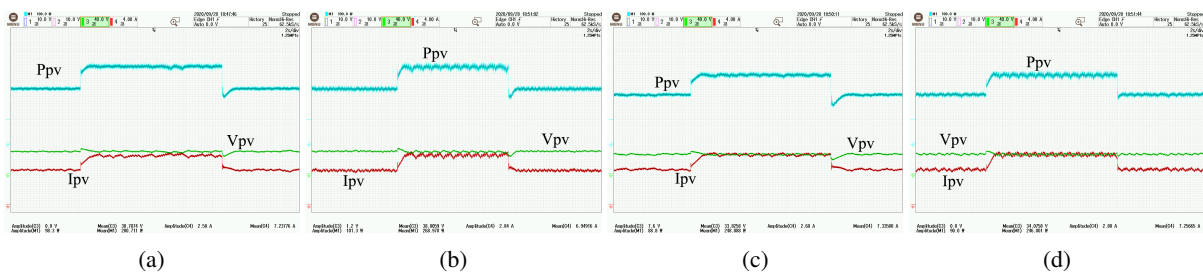
FIGURE 15: Experimental results : performance of proposed MPPT algorithm (a,c) and conventional P & O algorithm (b,d) under different irradiance pattern operating at 25^{\circ}C and 55^{\circ}C respectively
