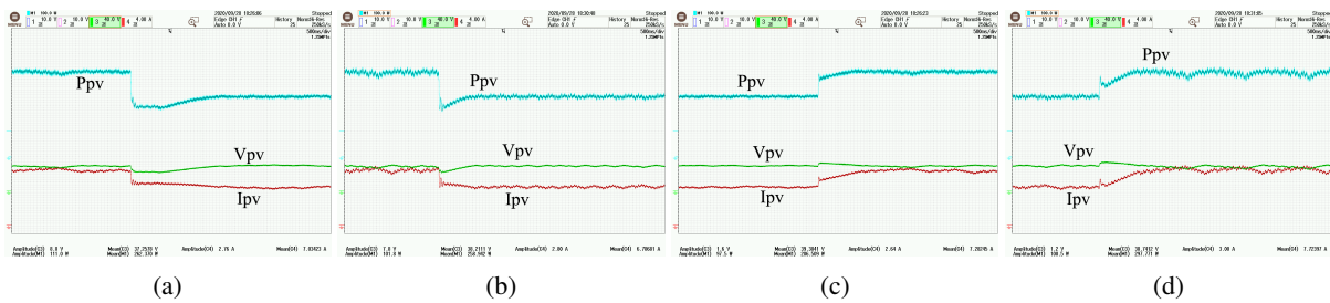
FIGURE 13: Experimental results : Sudden change in Irradiance operating at 25^{\circ}C (a,c) Proposed MPPT algorithm, and (b,d) Conventional P & O algorithm
