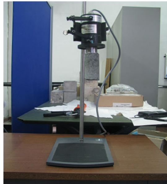
Fig. 2 The Luserna Stone specimen connected to the ultrasonic horn. The ultrasonic apparatus (Bandelin HD 2200) consists of a generator that converts electrical energy to 20 kHz ultrasound, and of a transducer that switches this energy into mechanical longitudinal vibration of the same frequency
