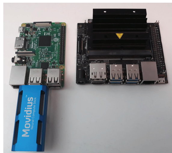
Figure 3: RPi 3B+ with Intel Movidius NCS on the left and NVIDIA Jetson Nano on the right
