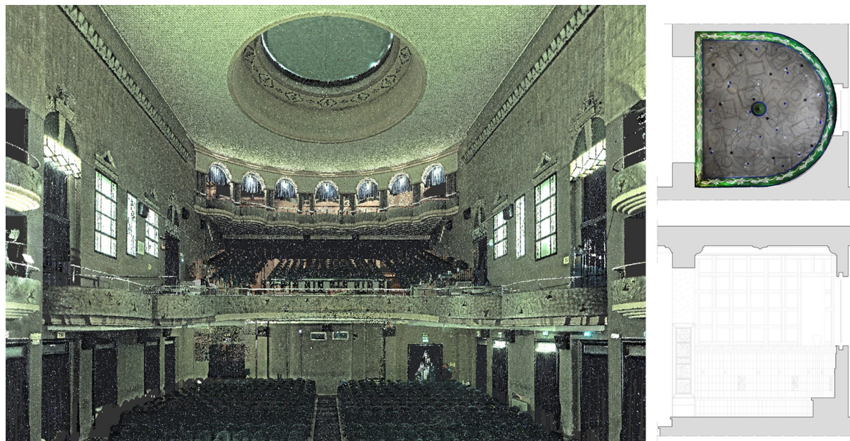
Figure 8. Cinema Odeon: (On the left) Perspective view of the TLS Point Cloud; (on the right) section and orthographic view of the lounge (restitution by Azzaro, Ciccia, Milici, Segreto, Tomasello, Zeremo)
