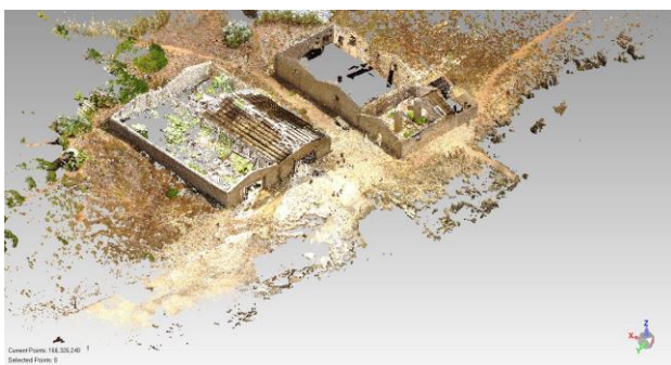
Figure 8. Point cloud model of the tonnara buildings on Capo Passero Island.
