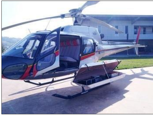
Figure 1. CNR IRPI aerial LiDAR mounted on EUROCOPTER AS350-B2
