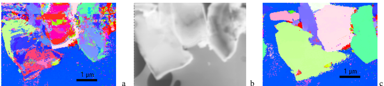
FIG.7 (a) Orientation mapping of mayenite crystals without precession (b) virtual bright field and (c) orientation map obtained with precession angle of 0.35^\circ
