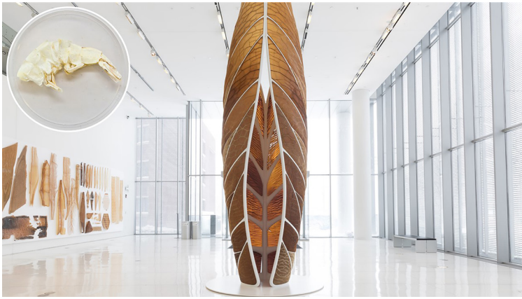
Fig. 2 Aguahoja I . Demonstrative pavilion developed using 3D printing biomaterials, mainly cellulose, chitosan, and pectin. Shape and material composition were guided by physical properties, environmental conditions, and fabrication constraints. Authors: J. Duro-Royo, L. Mogas-Soldevilla, D. Lizardo, J. VanZak, Y. Tai, A. Ling, C. Bader, N. Hogan, B. Darweesh, S. Sharma, J. C. Weaver, N. Zilberman, [...] and Prof. Neri Oxman. Elaboration of: https://oxman.com/projects/aguahoja
