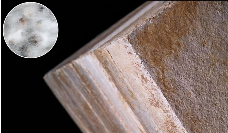
Fig. 3 Mycelium bricks . Biomaterial developed by Biohm company and used in construction, it can sequester about 16 tonnes/monthly of carbon. Authors/Credits: Biohm company. Elaboration of: https://www.micropia.nl/en/discover/microbiology/mycelium/ and https://www.biohm.co.uk
