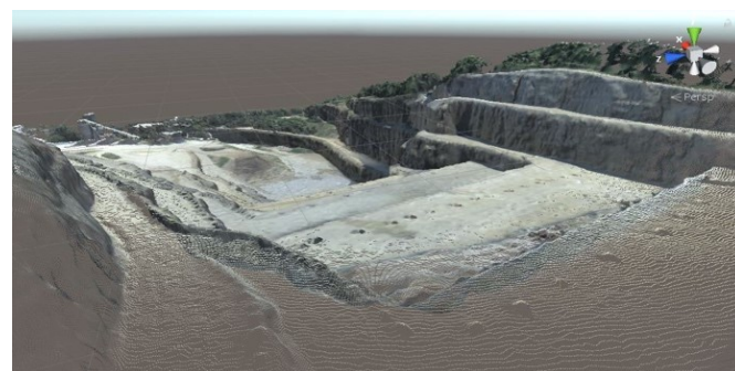
(c) Point cloud obtained projecting the pixels of the 360° image on the raw 3D mesh (Unity Software).
