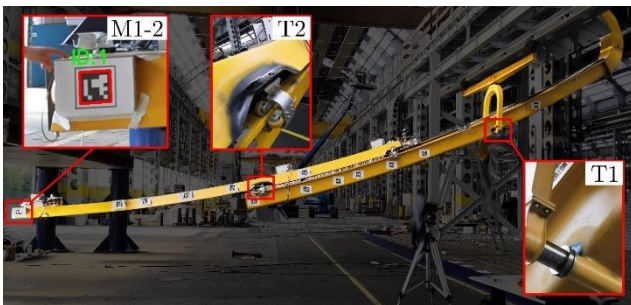
Figure 4. Tested CFRP structure: T1) First TSA analysed area; T2) Second TSA analysed area; M1-2) ArUco marker detected.
