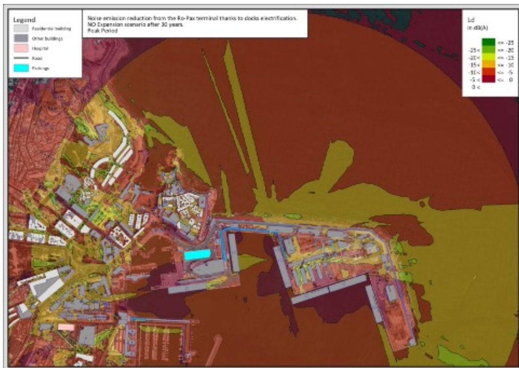
Figure 7: Effect of dock electrification of the Ro-Pax terminal: No expansion, 30 years, Peak season day period
