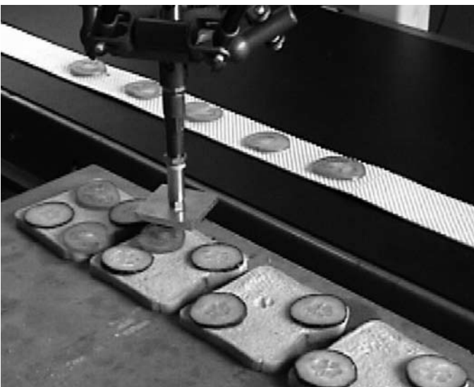
Figure 4 – Gripper mounted on robot.
